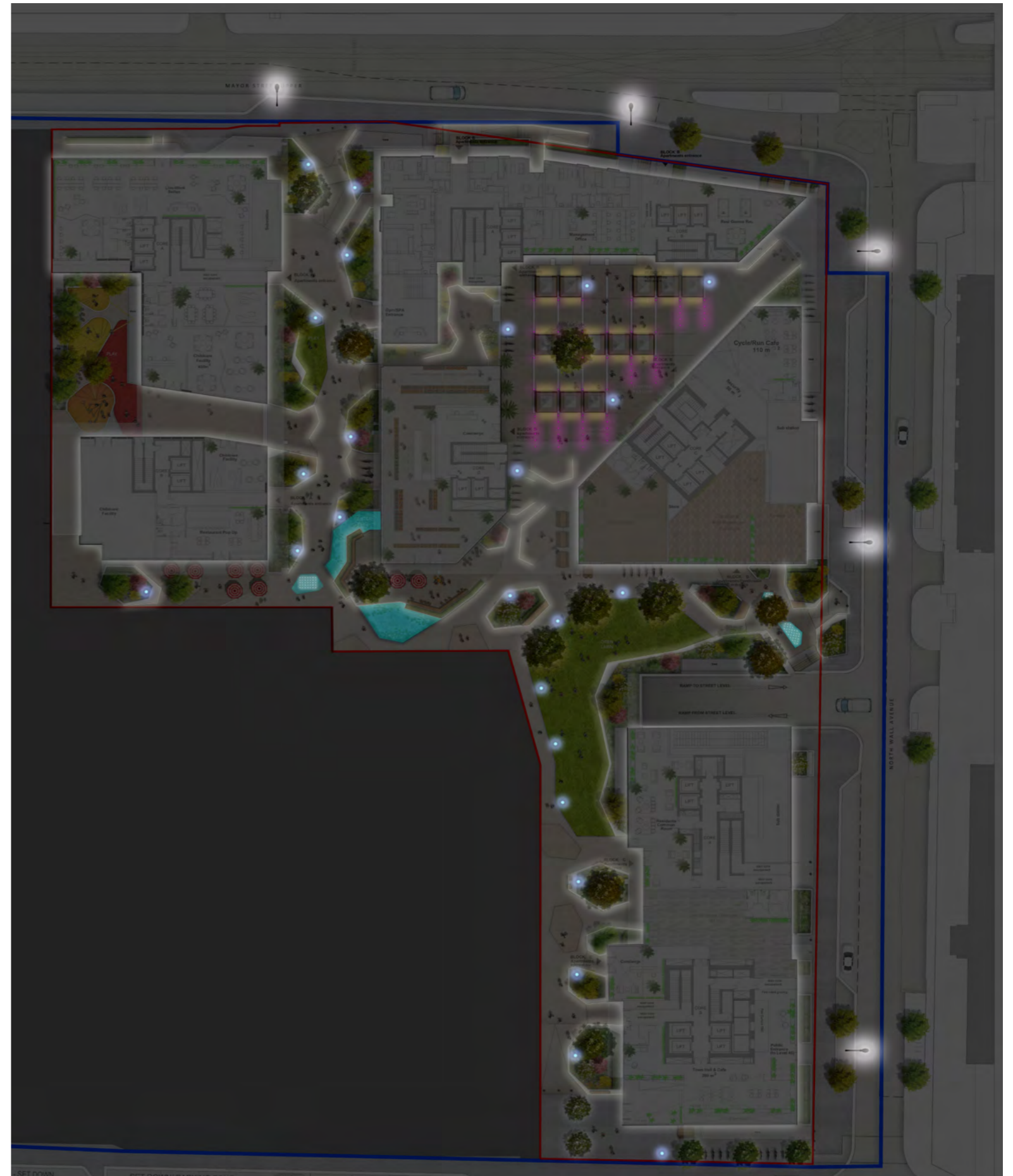
DCC Public Realm Lighting .: CitySoul gen2 LED Large Supplier: Philips or similar approved. Type: Brook Maxi 6m high, 24w led 36w with street optic. Colour: To match architectural metalwork.
