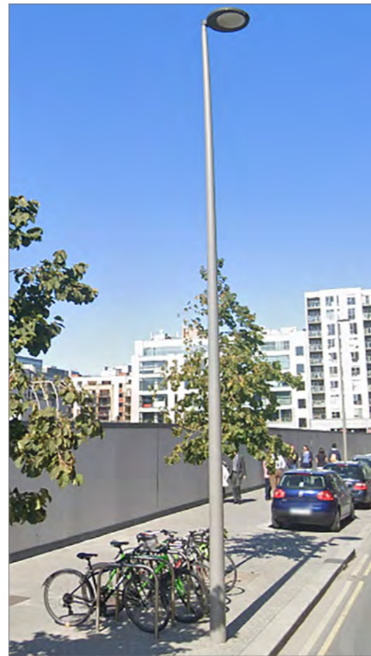
DCC Public Realm Lighting .: CitySoul gen2 LED Large Supplier: Philips or similar approved. Type: Brook Maxi 6m high, 24w led 36w with street optic. Colour: To match architectural metalwork.
